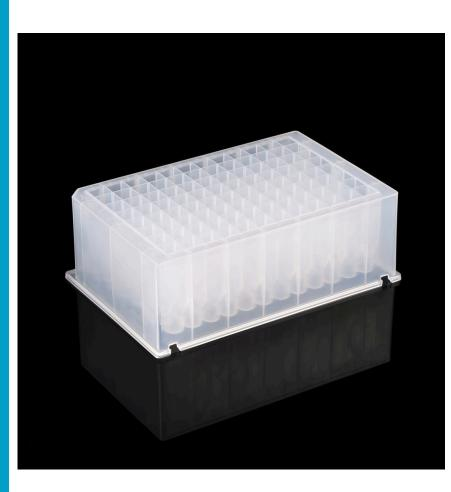
Designed for reliable DNA and RNA extraction in both research and clinical labs, this 96-well PCR plate is made from high-quality, DNA|RNA-free polypropylene. Each 2.0 ml well ensures durability and resists deformation across a temperature range of -20°C to +100°C, making it ideal for various thermal applications.
